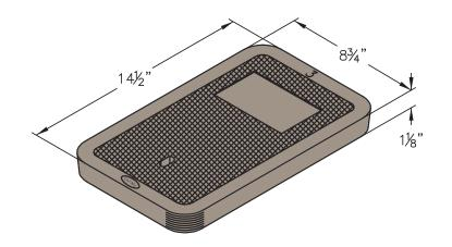
Style: Flush Material: Reinforced Concrete 9" x 14" Model: 12 lbs Weight: Options: Special Markings Surface: Skid Resistant & Marked\* Coefficient of Friction: >0.6 ASTM 1028 Performance: ASTM C 857, WUC 3.6
